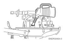
Use only high quality 4-stroke engine oil to insure performance and prolonged engine life.
