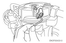
Remove the bolts (5pcs) and remove the recoil starter.
