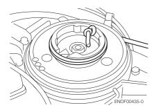
Tie a loop in the another end of the emergency starter rope and attach socket wrench that is included in the tool kit.
