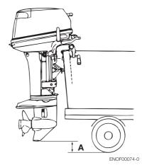
**A.** Ground clearance should be provided sufficiently. ENOW00073-0
