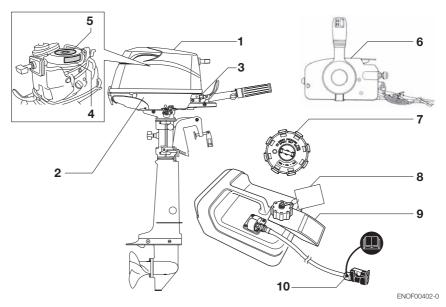
1. Warning label regarding owner's manual, top cowl, engine stop switch, engine oil level and unleaded gasoline.
