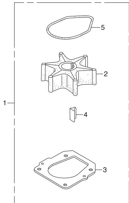
FOP-10-1 WATER PUMP IMPELLER KIT (2)
