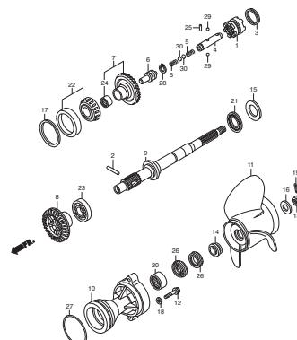
F-5-1 PROPELLER SHAFT/PROPELLER (XCA)
