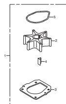
FOP-10-1 WATER PUMP IMPELLER KIT (2)
